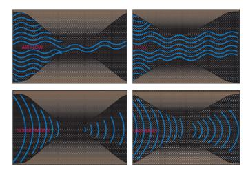
Because of this phenomenon, any unsealed gaps and clearances in door assemblies effectively cancel out the noise reduction benefits of sound doors. Hence, these unsealed gaps and clearances are required to be sealed with tested/certified Acoustical Gasketing.
