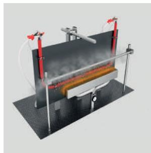
This test is carried out to verify circuit integrity during a fire. The cable is exposed to a flame at 830°C and mechanical shocks for 15 minutes and additional 15 minutes to flame, mechanical shocks and water spray.
