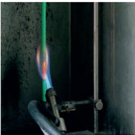
A 60 cm long sample of cable is vertically fixed with two clamps inside a small cabin, open on the front. The cable is subjected to the action of a flame produced by a calibrated Bunsen burner. The application time of the flame is according to the cable diameter (60-480 seconds). At the end of the test the burnt portion of cable must not be 50 mm close to the higher clamp.
