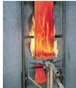
Samples of cables 3,5 m long in quantities required by standard are installed on a ladder inside a metallic cabinet. They are subjected to the action of a flame at 750°C for a specific time (20 or 40 minutes). Cables must not burn for more than 2,5 m.
