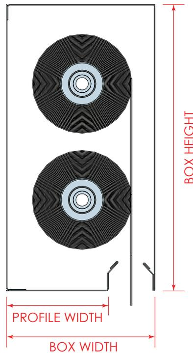
Multiple roller arrangement is for curtains of unlimited widths and for heights upto 6 meters under BSEN standards and upto 10 meters under UL standards.
