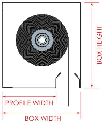
Single roller headbox can be provided for widths upto 6 meters and for heights upto 9 meters, while maintaining small sizes of head box which can be mounted in various methods.
