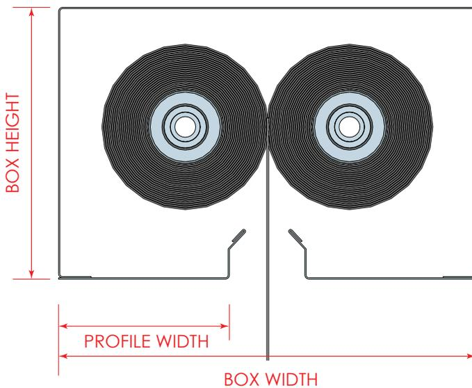
Multiple roller head boxes are also available in side by side configuration as shown in the figure. These arrangements are preferred for requirements where the height of the box (BH) need to be kept minimal.
