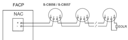
Figure 4. Wiring Diagram with FACP
