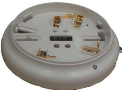
The 4098-9793EA IDNet Communications Isolator Base provides Simplex TrueAlarm analogue sensor operation and also provides IDNet communications isolation to improve installation convenience and increase system integrity. Isolation is automatically activated at the base when an output short circuit is detected and isolation can also be selected per base manually from the control panel to assist with troubleshooting wiring problems.
