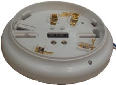
The TrueAlarm detector base contains integral addressable electronics that constantly monitors the status of the detachable detector. Detector types can be easily interchanged to meet specific location requirements, for example during building construction or maintenance. The base mounted address selection allows the address to remain with its programmed location when the detector is removed for service. An integral red LED indicates power-on by pulsing, or alarm or fault when steady on.
