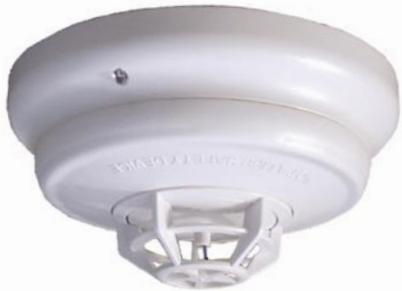
TrueAlarm heat detectors provide rate compensated, fixed temperature sensing, selectable with or without rate-of-rise temperature sensing. Due to its small thermal mass, the detector accurately and quickly measures the local temperature for analysis at the c.i.e. Rate-of-rise temperature detection is selectable at the c.i.e. Fixed temperature sensing is independent of rate-of-rise sensing. Configurable for either Type A or Type B as per AS 1603.1.
